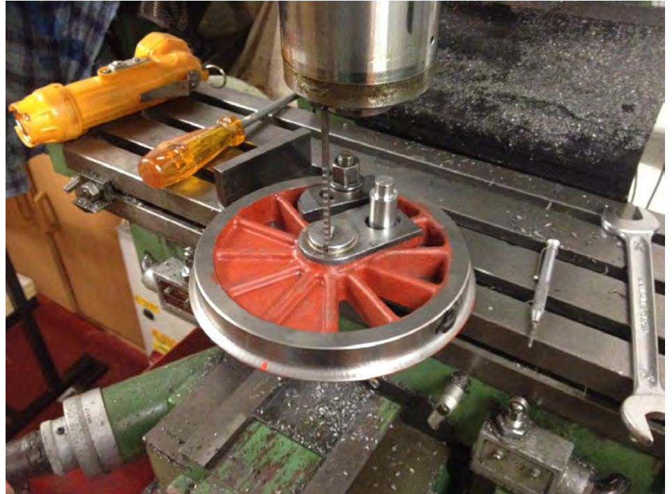
Wheels being broached using the miller as a press
