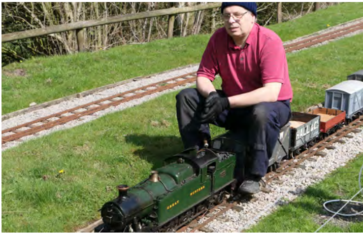
Vince Shaw, a member of GL5 and the Derby Society, scratch-built this 7200 Class 2-8-2T, N o 7243 from works drawings. The prototype was converted from a 2-8-0 around 1938 and it has an unusual backhead.
