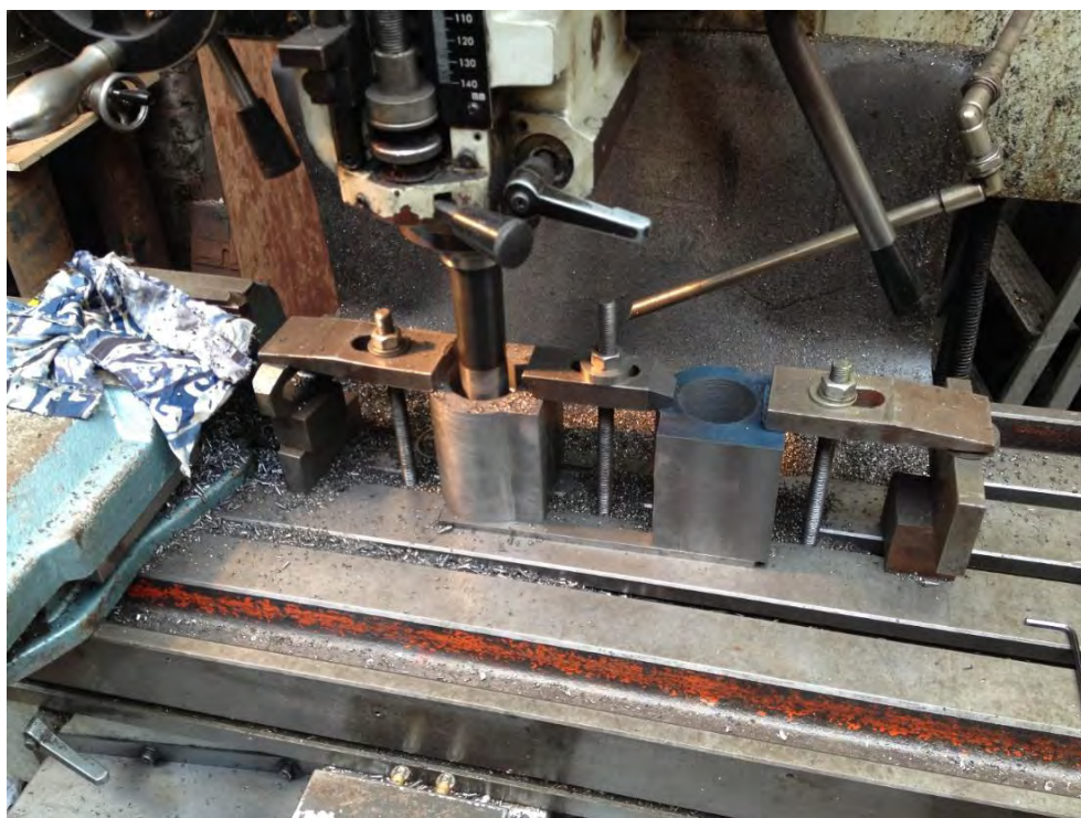
Cylinders being bored using a microbore (Note spacer under each cylinder so I didn't cut the table)
